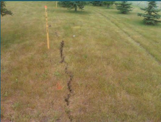
Note in the picture above the cracked soil resulting from over-pressurisation.
