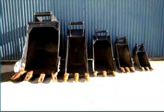
V-notched excavator trenching buckets such as the one pictured below (V-Raptor Bucket from Leading Edge Attachments) will help excavating a trench with sloped sides without over-excavating or disturbing the bottom.
